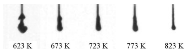
Figure 12. Photographs of solidified deposits remaining after the complete evaporation of UWS droplets for various ambient temperatures.
